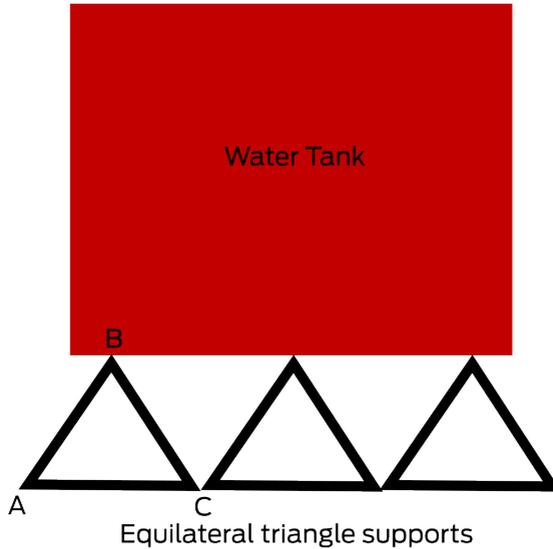
Assuming the weight is evenly distributed on the triangles, the compression force in AB is
