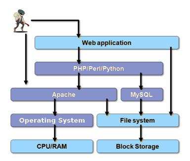
At each point in the diagram some kind of breach could occur with different tools and for different reasons.
